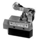
Enclosed Switches Series E6: Top Roller Arm Actuator, Adjustable with Steel Roller; 1NC 1NO SPDT Snap Action; 0.5 in - 14NPT conduit
